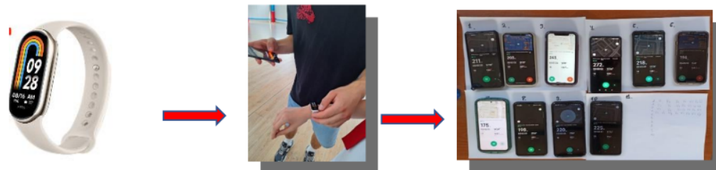
Figure 1. Connecting the Xiaomi 8 band watch to the MI Fit app and sending data to phones
